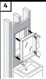
Cut the marked perimeter with appropriate tool.
