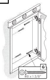
Level, then secure the medicine cabinet with the screws (G) through the mounting holes into the framing studs.
