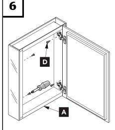
Attach mirrored side panels to the medicine cabinet using a screwdriver and provided screws (D).
